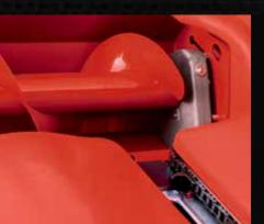
The feeder auger has a big diameter with crossing spirals. This guarantees an even and continuous material flow also under the most difficult conditions avoiding material losses. The auger is driven by a maintenance free gearbox in oil bath with an integrated slip clutch in a case made of a special aluminium alloy.
