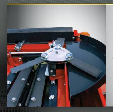
The stalk chopper is integrated in the row unit gearbox and not an add on. This provides a minimal power consumption providing an incomparable. Every stalk chopper can be switched off individually.
