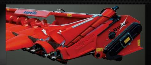
The optional fender auger is used for the harvest of down corn.
