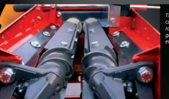
The profile and the construction of the knife rollers as well as the row uni gearbox are the heart of this evergreen corn head model.
